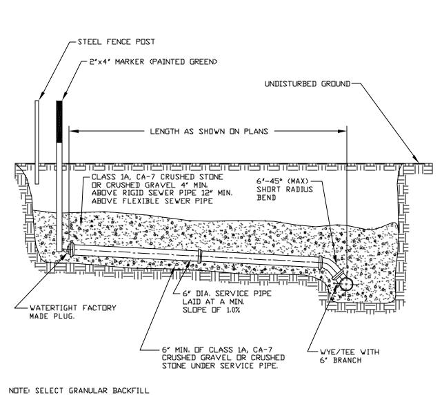
NOTE: SELECT GRANULAR BACKFILL REQUIRED UNDER PAVED AREAS BACKFILL TO BE APPORVED BY APPROPRIATE MUNICIPALITY.
